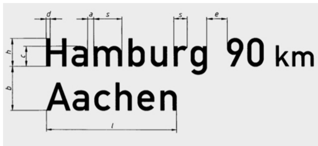
Rules and measurements from the DIN 1451-2 specification.
